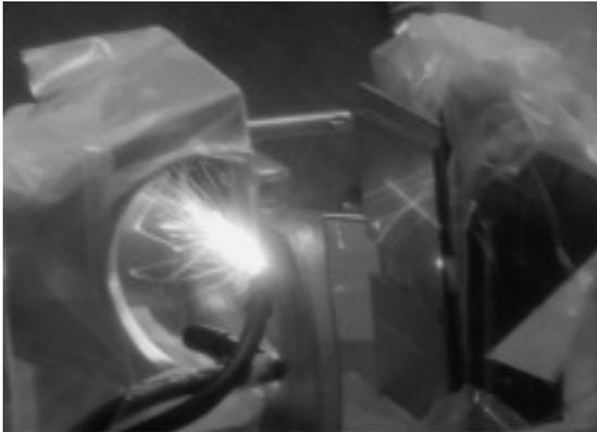
Fig. 14 High power laser lights irradiated surface of heavily-contaminated stainless-steel sample, and hot stainless-steel particles were evaporated from the high speed scanned spots during the 2013 March trial
