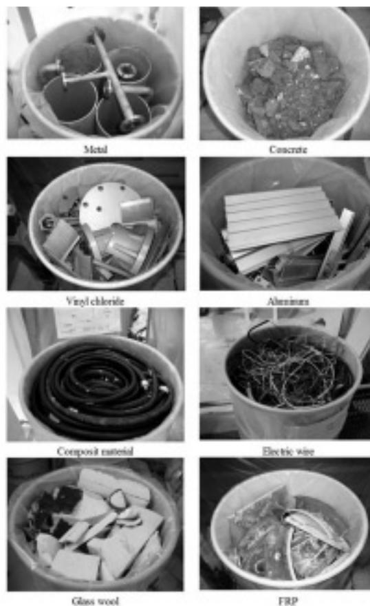
Photo 7 Typical material for dismantling
