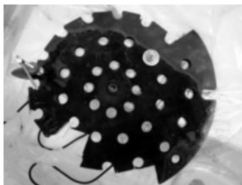
Fig.12 A large stainless-steel disk with many holes was used to make about 35mmx35mmx10mm rectangular and heavily RI-contaminated block samples for the 2013 March laser decontamination trial
