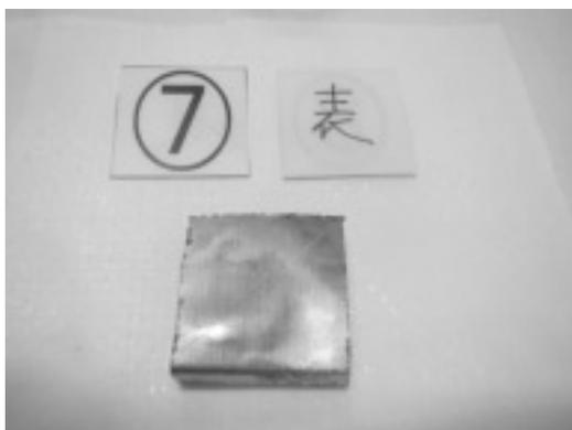
Fig.15 Shining surface of the stainless-steel sample (about 35mm x 35mm x 10mm) just after the laser decontamination
