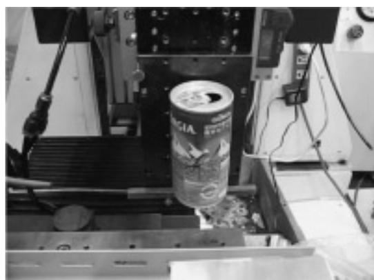
Fig. 6 Laser surface peeling of a coffee aluminum can
