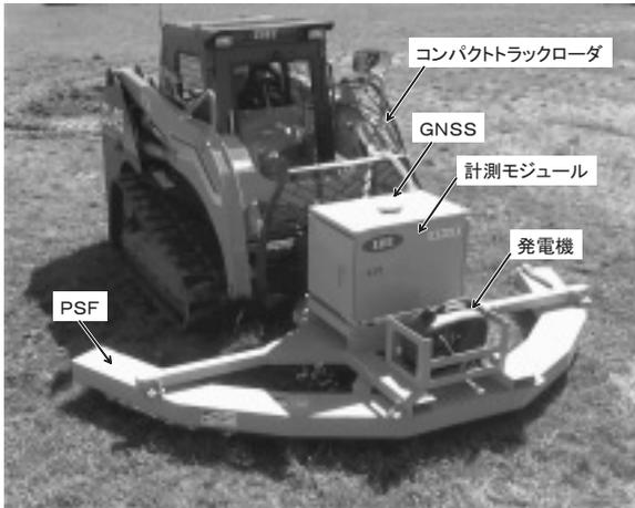
Fig. 2 Photo of radiation beam measurement system with PSF on compact track loader (CL45)
