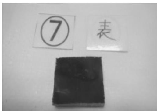
Fig.13 About 35mm x 35mm x 10mm rectangular and heavily RI-contaminated block samples before the laser irradiation
