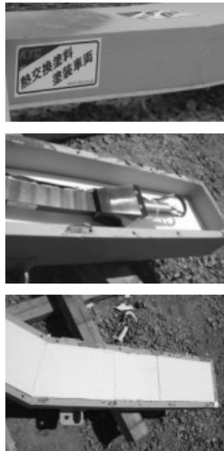
Fig. 3 Methods to prevent PSF from heating (Left: anti-thermal painting, centre, Right: heat insulator inside the PSF casing)
